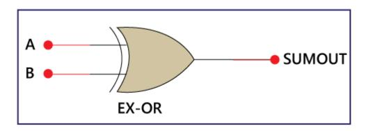
The above is the symbol of the **EX-OR** gate. In the above diagram, 'A' and 'B' are the inputs, and the 'SUMOUT' is the final outcome after performing the XOR operation of both numbers.
