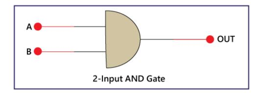
The above is the symbol of the **AND** gate. In the above diagram, 'A' and 'B' are the inputs, and 'OUT' is the final outcome after performing AND operation of both numbers.
